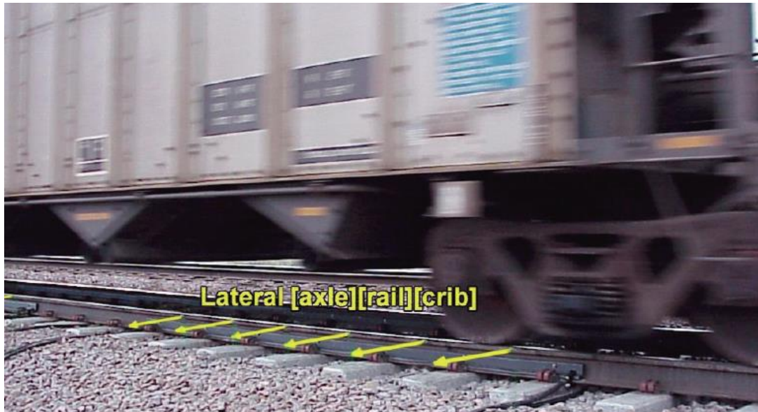
Figure 8: LBF/Salient Hunting Truck Detector (HTD)
