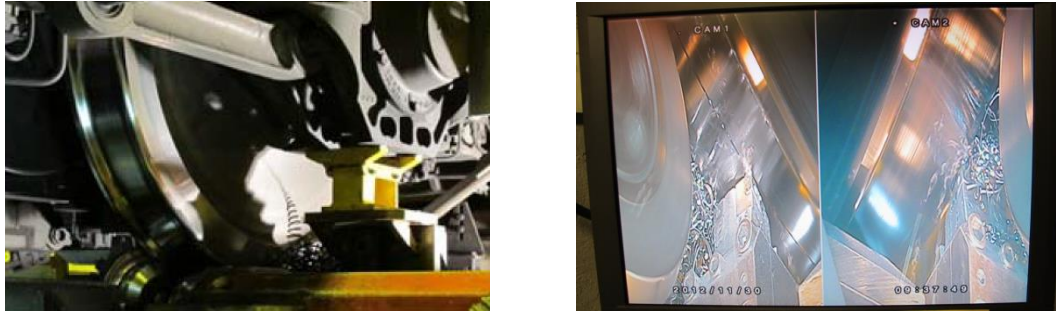
Figure 23 : Locomotive wheel-sets undergoing on-site re-profiling
