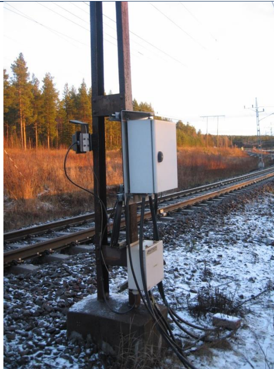
Figure 17: Minimal system cabinet that contains sensor electronics and optionally also computer and communication electronics.
