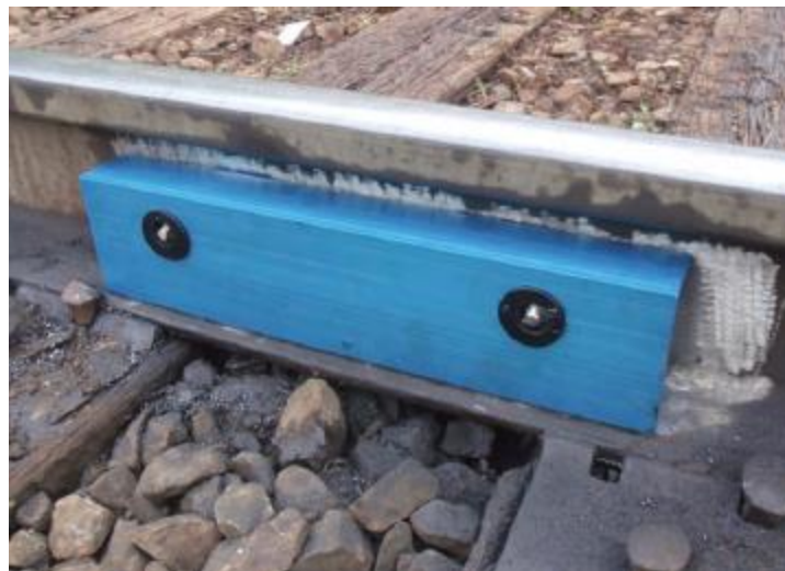
Figure 7: LBF/Salient Systems Wireless L/V Detector
